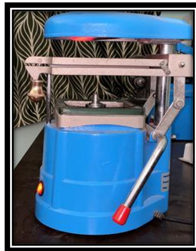
Fig. 5b: Vaccumforming Machine with master die in place
