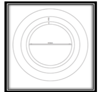
Fig. 2b: Stainless steel die with dimensions (frontal and top view)
