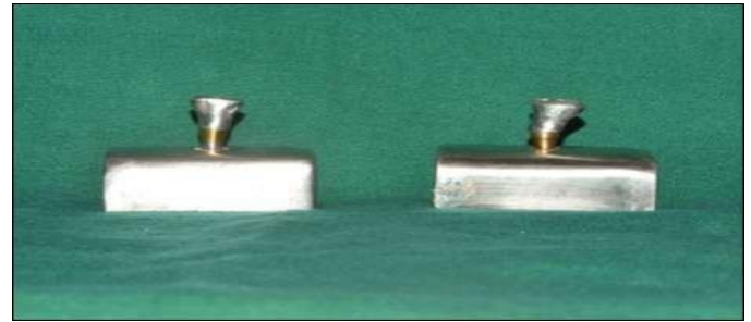
Figure 7: Implant abutment (4 mm gh) with metal mounting jig.
