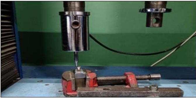
Figure 10: Application of cyclic loading with universal testing machine
