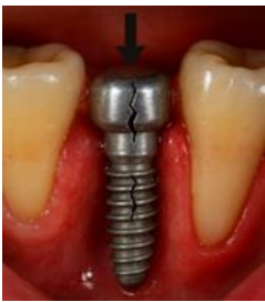
Figure 5: Fractured narrow implant under occlusal stress, highlighting mechanical limitations.
