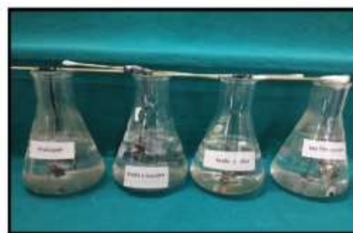
Figure 6: Samples hung in 10% Nitric acid for decalcification
