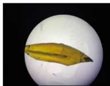
Figure 12: No Ink was removed. (Grade 3)
