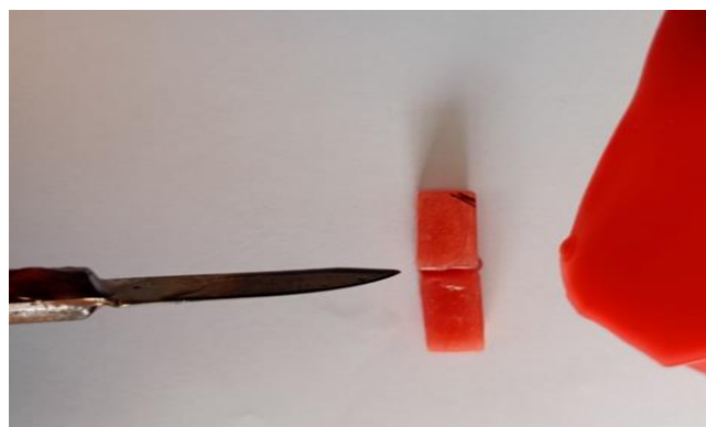
Figure 17: Baseplate wax is filled into the 3 mm space between two specimens
