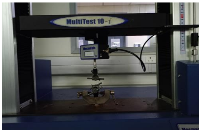
Figure 26: Samples loaded onto the universal testing machine
