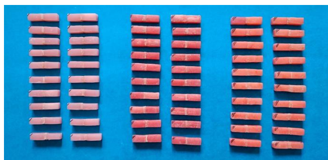
Figure 23: Pmma specimens with molloplast b incorporated between two blocks
