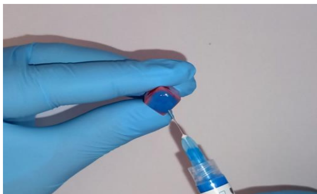
Figure 13: Surface treatment of specimens with 36% phosphoric acid
