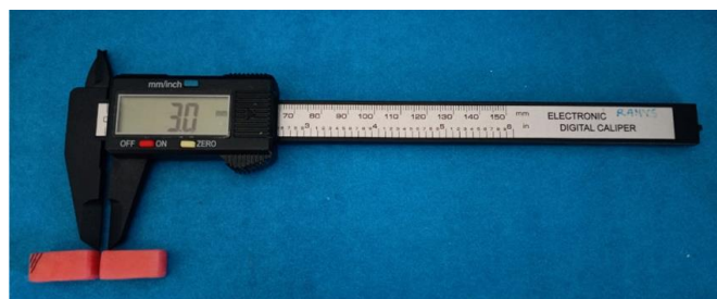
Figure 17: Baseplate wax is filled into the 3 mm space between two specimens
