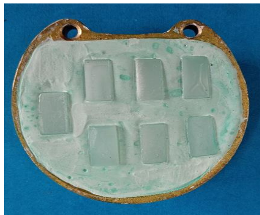
Figure 5: Mold Space after Dewaxing
