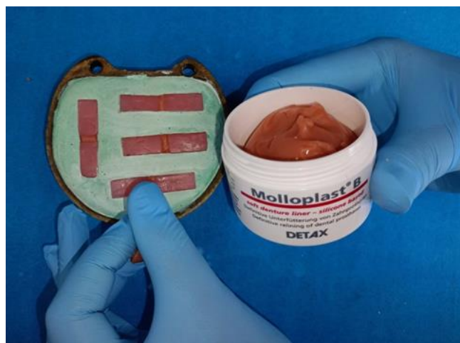
Figure 23: Pmma specimens with molloplast b incorporated between two blocks
