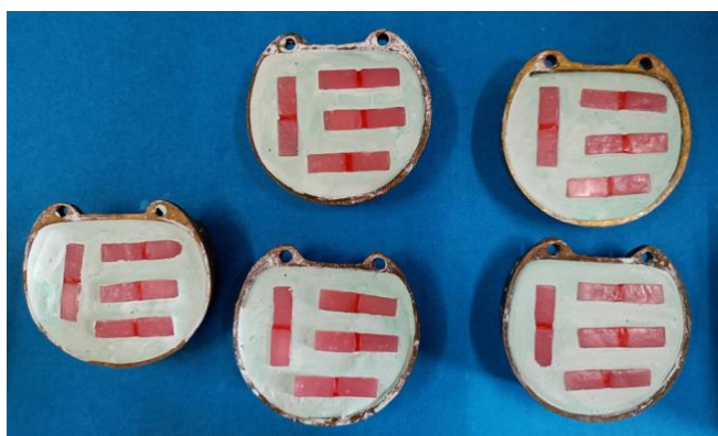
Figure 20: Dewaxing of samples was done
