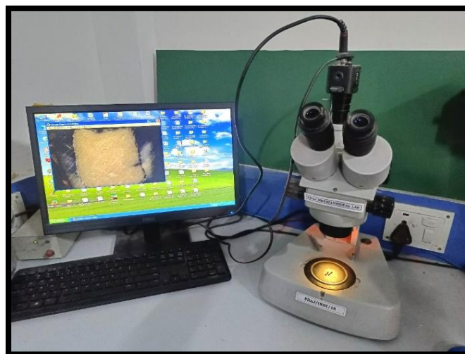
Figure 1: Each Sample Was Examined Under a Stereomicroscope At 10x Magnification.
