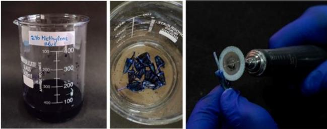
Figure 15: Immersion of specimens in 2% methylene blue & vertical sectioning of specimens using diamond disc
