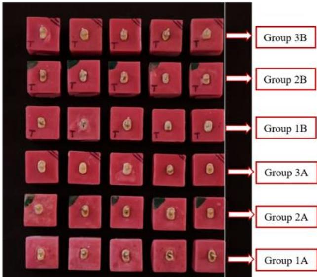
Figure 12: Specimens mounted in autopolymerising resin
