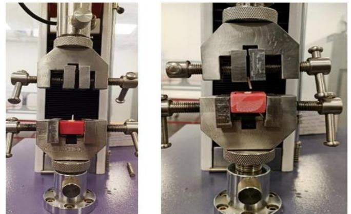
Figure 14: Testing for pull-out bond strength
