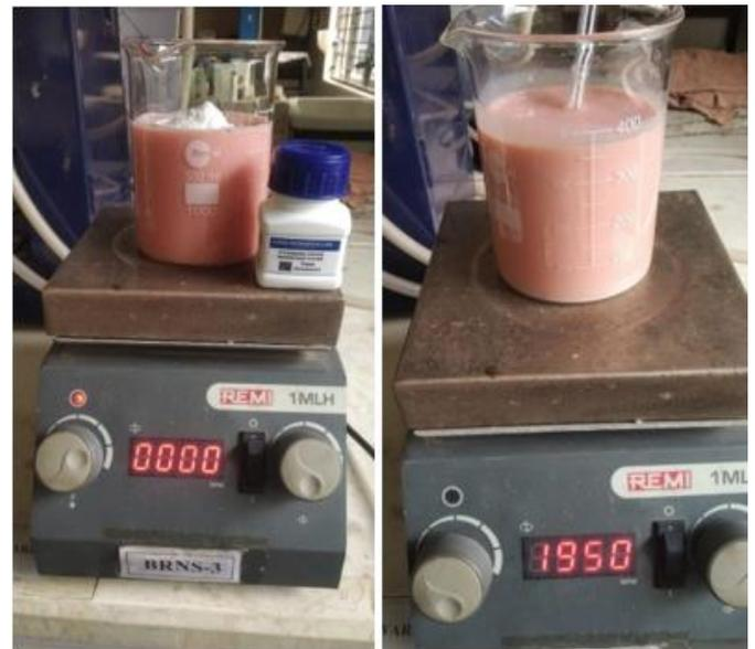
Figure 6: Resin with added TiO<sub>2</sub> nanoparticle was magnetically ultrasonicated stirred
