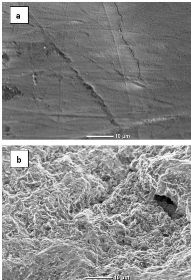
Figure 8: SEM images of resin a) without nanoparticles b) with TiO<sub>2</sub> nanoparticles
