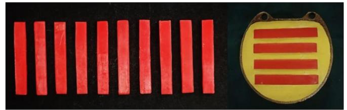
Figure 2: Wax pattern of the specimens before dewaxing
