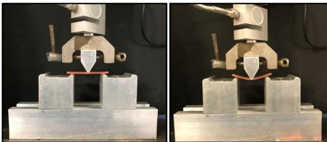
Figure 10: Flexural strength of the specimens tested using UTM
