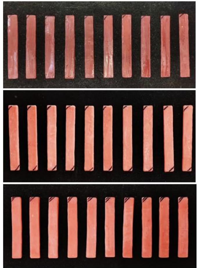
Figure 9: Group 1: heat polymerised PMMA specimens; Group 2: 3D printed denture base resin specimens; Group 3: TiO<sub>2</sub> nanoparticles incorporated in 3D printed denture base resin specimens
