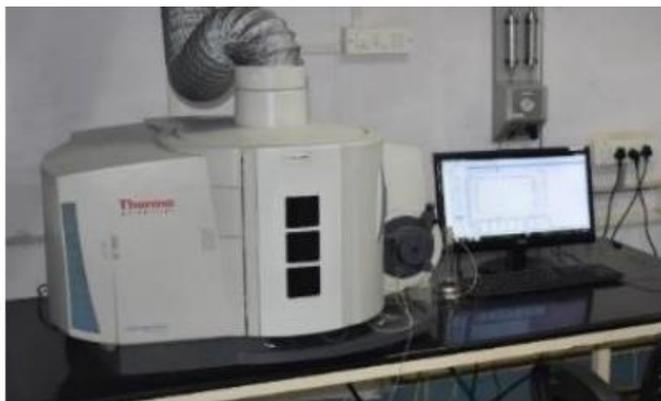
Figure 5: Inductive coupled plasma spectrometry
