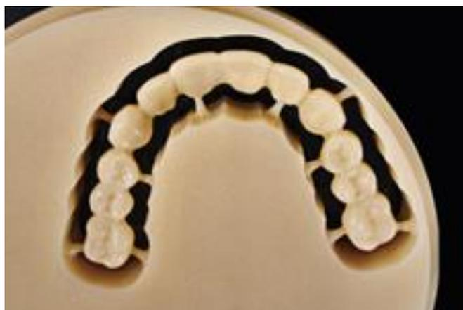
Figure 1: Milled teeth connected into single arch
