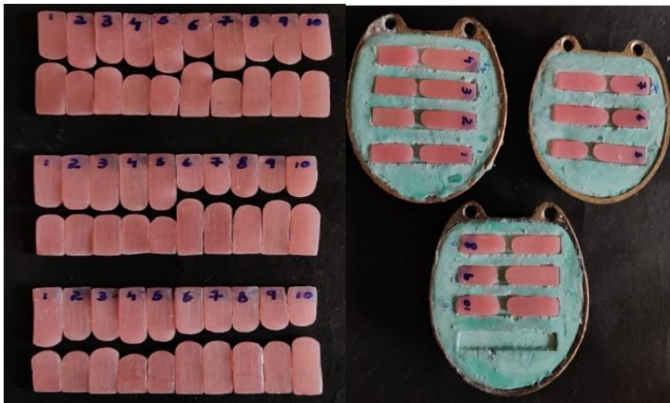
Figure 3: Fractured acrylic samples placed back into mould space.
