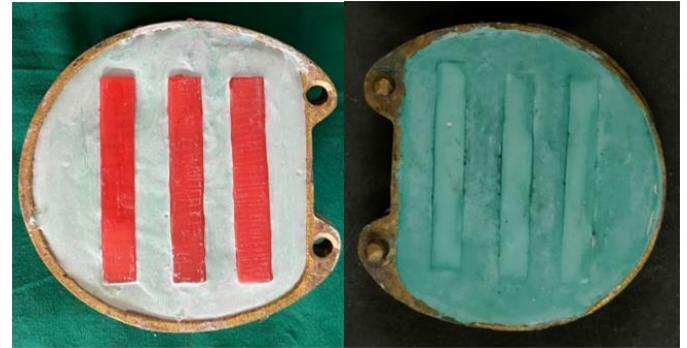
Figure 2: before and after dewaxing.
