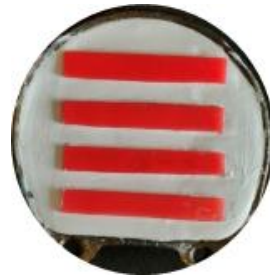
Figure 2: Wax samples invested in Plaster of Paris
