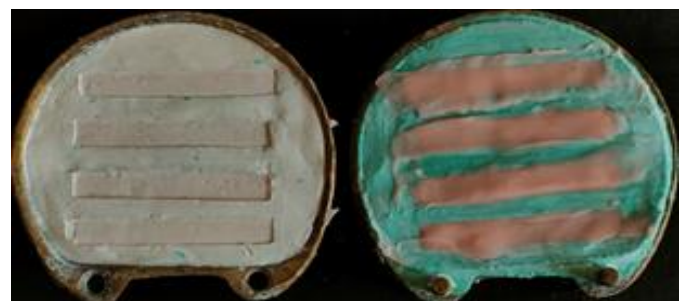
Figure 4: Conventional one step packing of unmodified PMMA for Group 1 .
