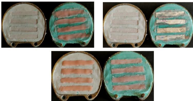
Figure 5: Double layer packing technique for Group 3.
