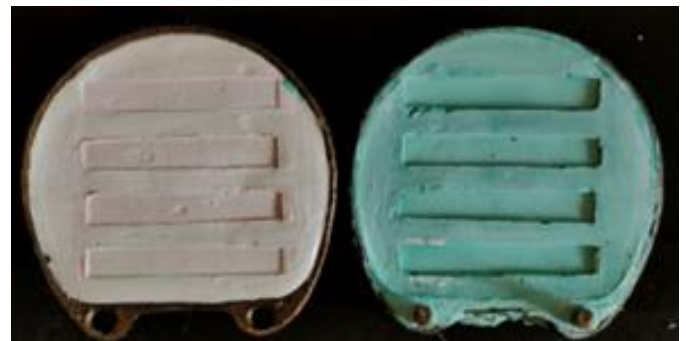
Figure 3: Mold space after dewaxing procedure
