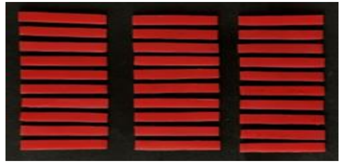
Figure 1: Preparation of wax specimens measuring 65mm×10mm×25mm.
