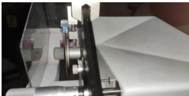
Fig.5 mesio-distal sectioning of specimens in microtome
