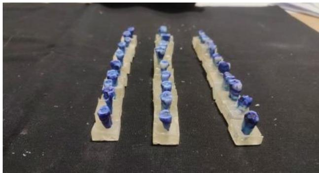
Fig.4 Dye penetration in methylene blue dye
