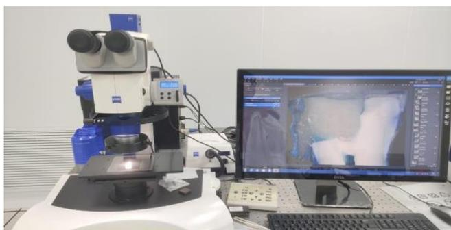
Fig. 6: Investigation of microleakage using stereomicroscope
