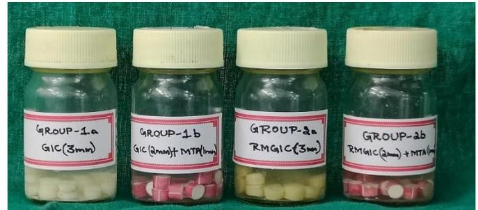
Figure 1: Single layered and bilayered GIC and RMGIC discs prepared and stored in artificial saliva prior to Vickers hardness testing.
