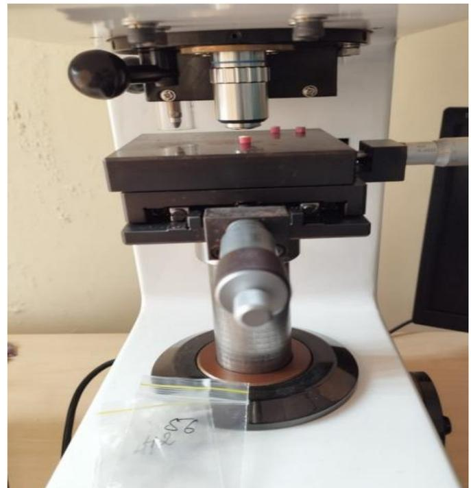
Figure 2: GIC and RMGIC discs being examined to assess surface microhardness on the Vicker's hardness testing machine (Micro Mach Technologies S1300)
