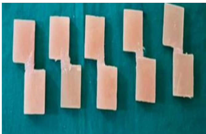
Fig 2: Acrylic Sample tested for Tensile strength in UTM.
