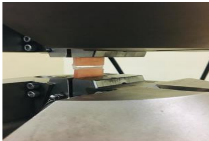
Fig 3: Acrylic Samples used for Shear strength testing.
