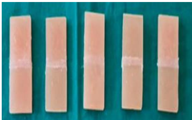
Fig 1: Acrylic Samples used for Tensile strength testing.
