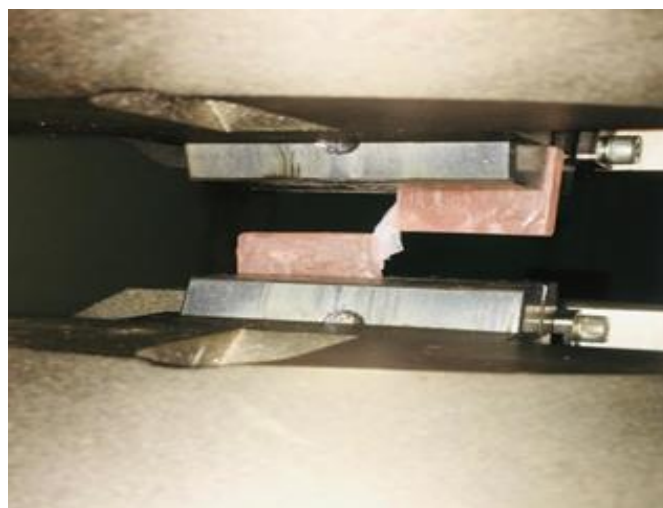
Fig 4: Acrylic Sample tested for Shear strength in UTM.
