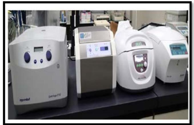
Figure 8: Major Centrifuges used for PRF preparation.
