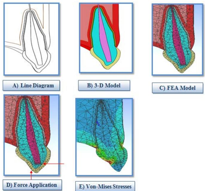
Figure 1: Creation of Geometric Model, FEM Model and Force Application
