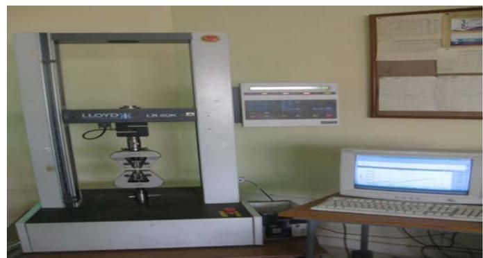
Figure 4: Universal Testing Machine (Instron)
